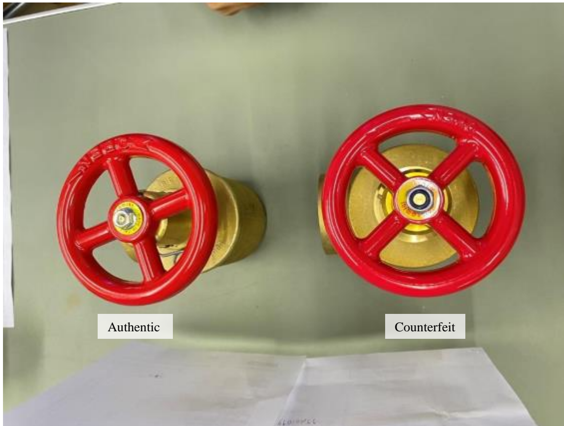
Figure 2. Photograph of an authentic Giacomini SpA, A155 pressure restricting valve (left) and a counterfeit A55 pressure restricting valve (right). The Giacomini SpA handle ring is yellow in comparison to an orange handle ring on the counterfeit pressure restricting valve.
