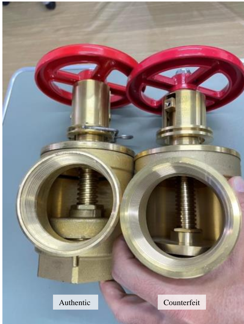
Figure 1. Photograph of an authentic Giacomini SpA, A155 pressure restricting valve (left) and a counterfeit A55 pressure restricting valve (right). Internal differences include a smaller internal shutter on the A55 valve and loose engagement of the stem on the bonnet.
