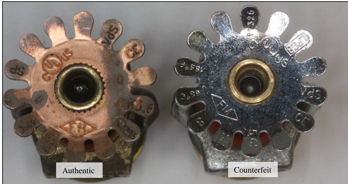
Figure 4. Authentic TY325 deflector (left) and counterfeit deflector (right). The markings are similar, including the appearance and position FM Approvals mark.
