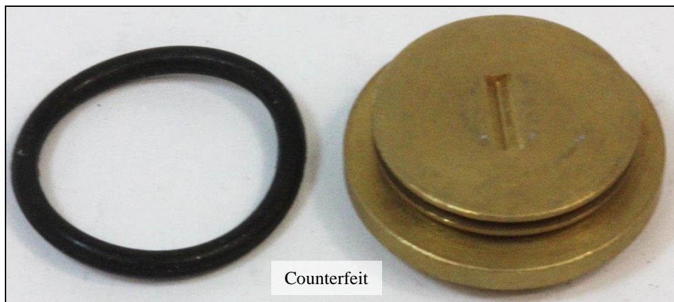
Figure 3. Counterfeit TY7226 sprinkler seal. The counterfeit cap superficially resembles the authentic version but conceals a potentially unreliable O-ring type seal.
