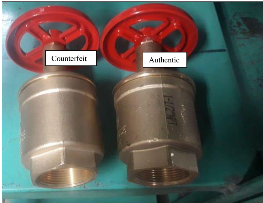
Figure 4. The side of the valve bodies opposite the outlets of both the counterfeit (left) and authentic valve (right). There is a line of laser print on the body of the authentic valve indicating the nominal pipe size and thread standard “1-1/2”NPT” that does not appear anywhere on the counterfeit valve.
