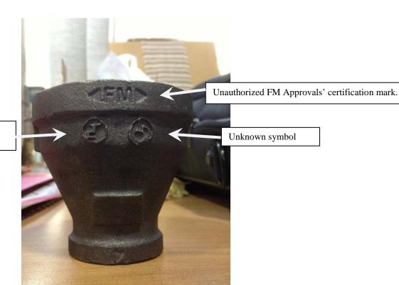
**Figure 1** – Example of the marking identifiers on the counterfeit castings.
