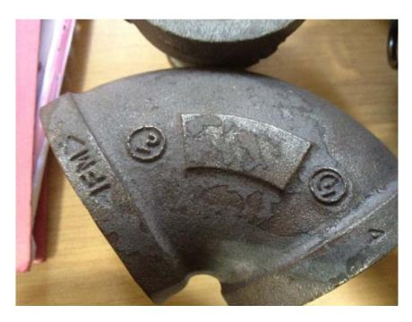
**Figure 2** – Second example of counterfeit casting. Note the same identifiers as Figure 1.
