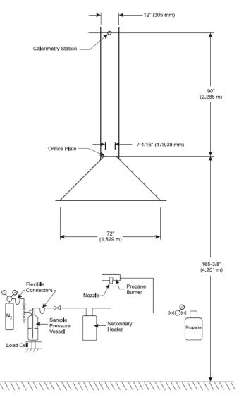
FM Heat Release Rate Measurement Apparatus
