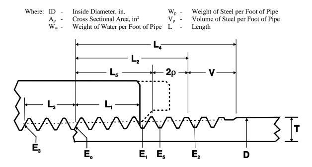
Establish the pitch diameter at the pipe end  $(E_0)$  for NPS 2 (DN 50) Schedule 40 pipe:
