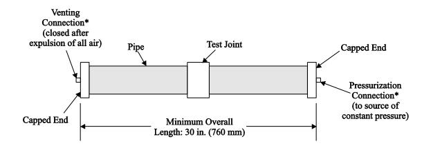
\*End caps shall be drilled and tapped to 3/8 or 1/2 inch NPT in order to make use of standard connectors. Manufacturer to supply connectors if other than NPT.
