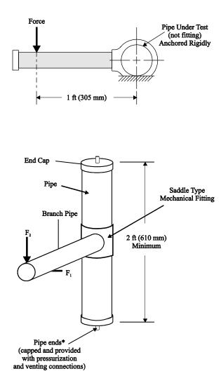
\*End caps shall be drilled and tapped to 3/8 or 1/2 inch NPT in order to make use of standard connectors. Manufacturer to supply connectors if other than NPT. Figure C-4. Vibration Test
