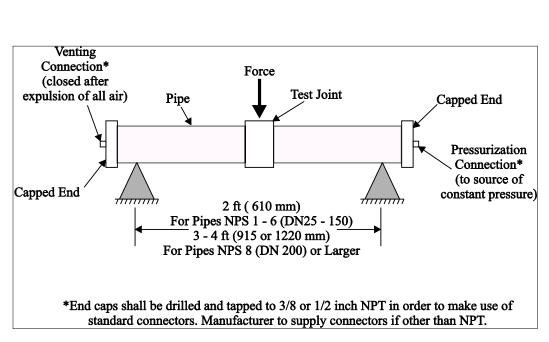
Figure C-2. Bending Moment Test
