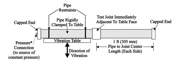
\*End Caps shall be drilled and tapped to 3/8 or ½ inch NPT in order to make use of standard connections. Manufacturer to supply connectors if other than NPT.
