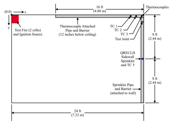
Figure 4.5.2 – Set-Up for Fire Test 4.5
