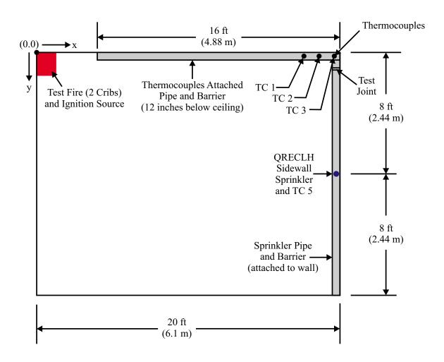
Figure 4.4.2 – Set-Up for Fire Test 4.4
