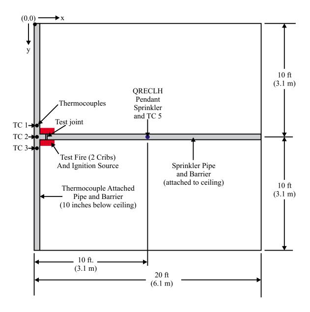
Figure 4.2.2 – Set-Up for Fire Test 4.2 and 4.3
