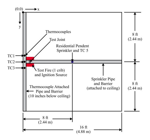
Figure 4.6.2 — Set-Up for Fire Test 4.6
