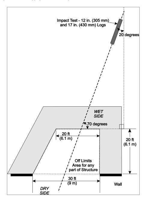
Figure 4.2.5.2 Debris Impact Test Layout
