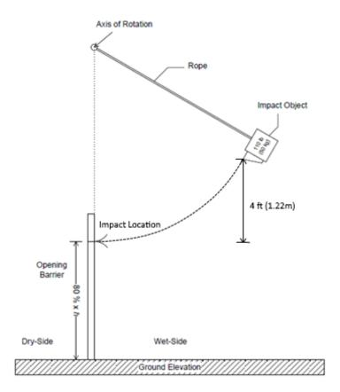
Figure 4.3.4 Impact Test Layout
