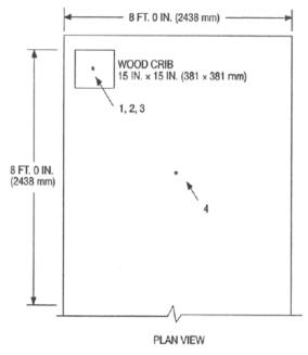
Figure C-3.1 Thermocouple locations
