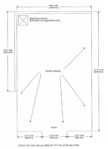
Figure C-2. Plan view of Test Room
