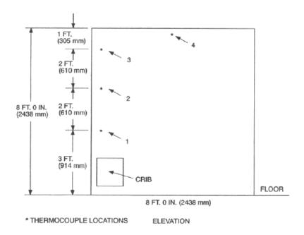
Figure C-2.2 Thermocouple locations
