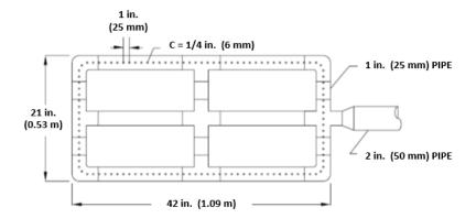
Figure D.2 - Top view of pipe burner
