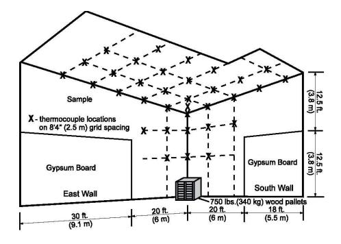
Figure E.1 25ft (7.6 m) Corner Test Structure
