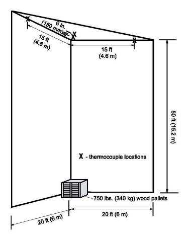
Figure F.1 50 ft (15.2 m) Corner Test Structure
