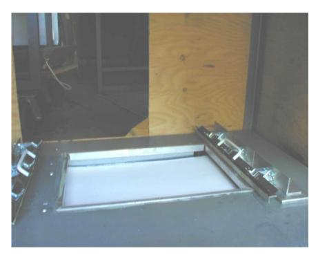
Figure B-7. Paper Tray Below Welding Pad or Blanket – Paper Ignition Test.
