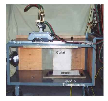
Figure B-1. Welding Pad, Blanket and Curtain Test Apparatus.
