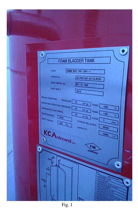
This photo of the counterfeit tank was taken by the third party installing firm at the location to which the counterfeit tank was shipped. Distinguishing characteristics of the counterfeit product include the incorrect font that appears in the K. C. Antincendi logo.
