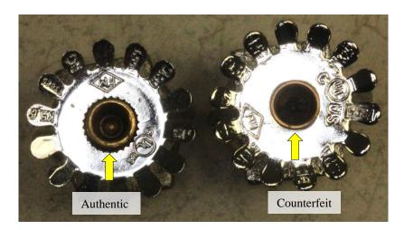
**Figure 3.** Authentic TY325 deflector (left) and counterfeit deflector (right). The markings are similar, including the appearance and position of the FM Approvals mark. The yellow arrows indicate the different appearance of the deflector attachment.
