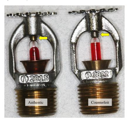
**Figure 1.** Photograph of an authentic Tyco TY325 sprinkler (left) and a counterfeit TY325 sprinkler (right). The arrows highlight the different appearing compression screws.
