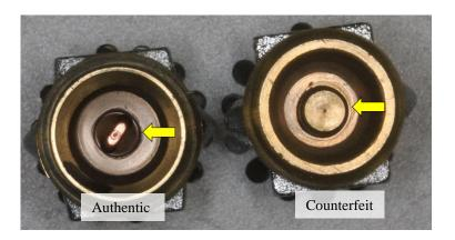
**Figure 2.** Authentic Tyco sprinkler (left) and counterfeit (right). The bottoms of the orifice caps are indicated by the yellow arrows.
