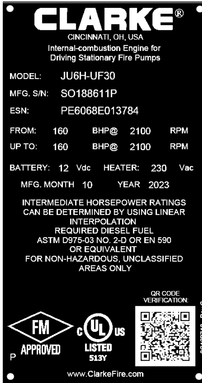
Figure 2. Photograph of an actual Clarke Fire Protection Products nameplate with a QR code. The QR code links to a Clarke Fire Protection Products website where a user can validate a product's data.
