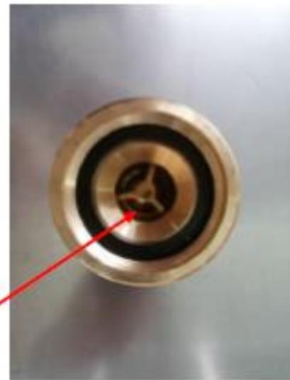
**Figure 2:** Counterfeit A7 1-1/2" Firehose Nozzle (Bottom View) – Shape of the internal support is different as displayed by red arrows.
