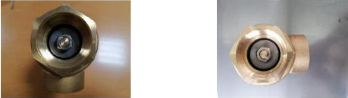
**Figure 6:** Counterfeit A55 1-1/2” Standard Hose Valve (Bottom View) – The nut on the counterfeit valve is made of carbon in comparison to stainless steel which is in accordance with requirements on the actual valve.
