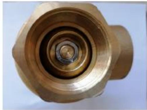
**Figure 9:** Counterfeit A155 1-1/2" Pressure Restricting Valve (Bottom View) - The nut on the counterfeit valve is made of brass in comparison to stainless steel nut on the actual valve.
