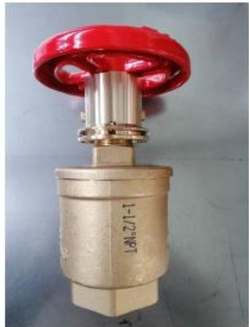
**Figure 8:** Counterfeit A155 1-1/2" Pressure Restricting Valve (Side View) - The thread type is printed on the body of the actual valve.
