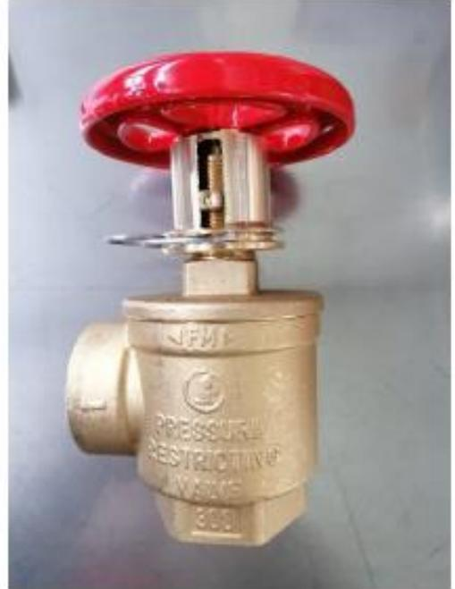
**Figure 7:** Counterfeit A155 1-1/2" Pressure Restricting Valve (Front View) - the counterfeit products are illustrated by the images on the left while the examples on the right are the actual FM Approved products. Counterfeit valve has incorrect designation "Pressure Reducing Device" on the cast valve body.
