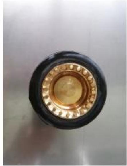
**Figure 3:** Counterfeit A7 1-1/2" Firehose Nozzle (Top View) – The machining of the teeth on the counterfeit nozzles are irregular (randomly squared, trangular, etc).
