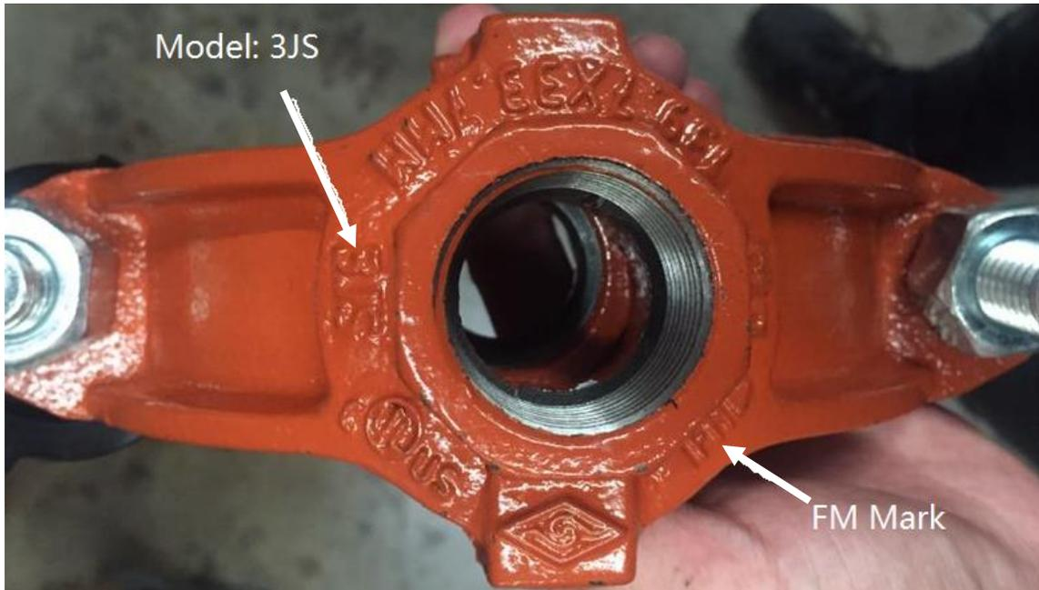
**Figure 2.** Top view of one of the products shipped as the Model 4JS mechanical cross, incorrectly showing the Model 3JS marking.
