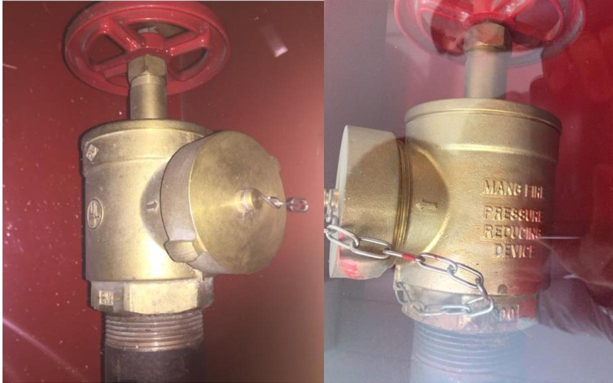
**Figure 2 – Suspected Counterfeit Angle Hose Valve**
