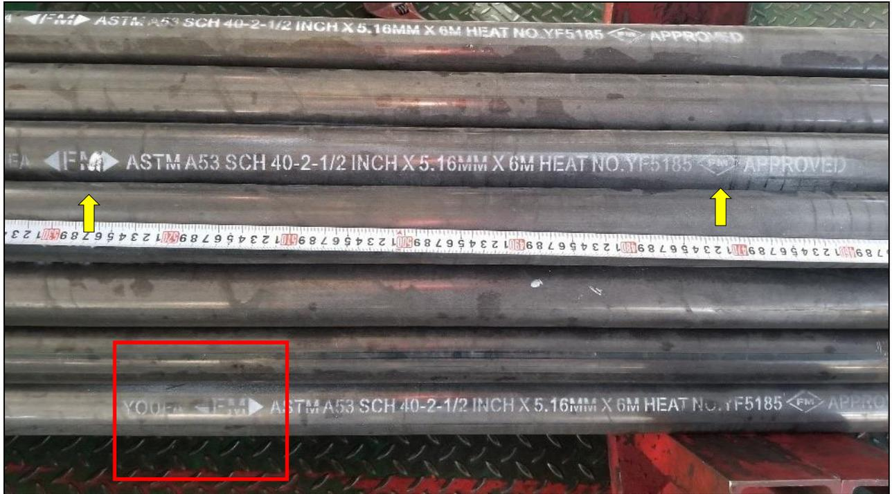
**Figure 1.** Steel pipe from Youfa marked with two versions of counterfeit FM Approvals markings
