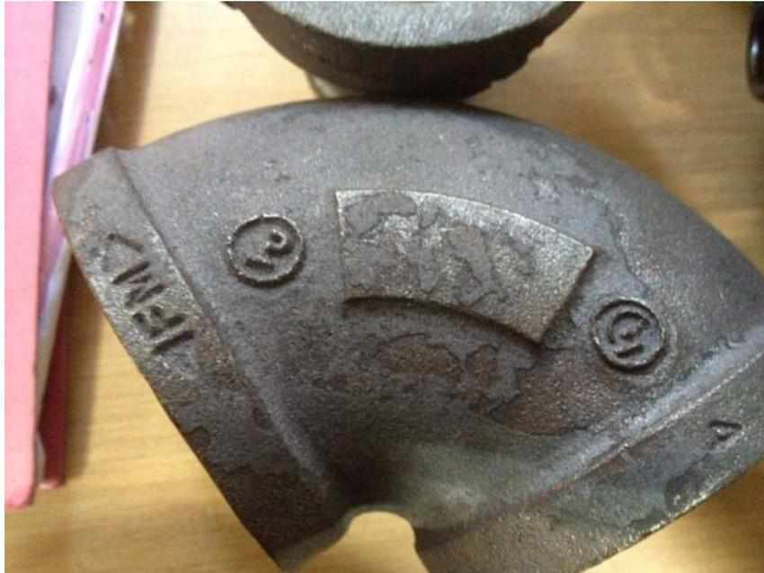
**Figure 2** – Second example of counterfeit casting. Note the same identifiers as Figure 1.
