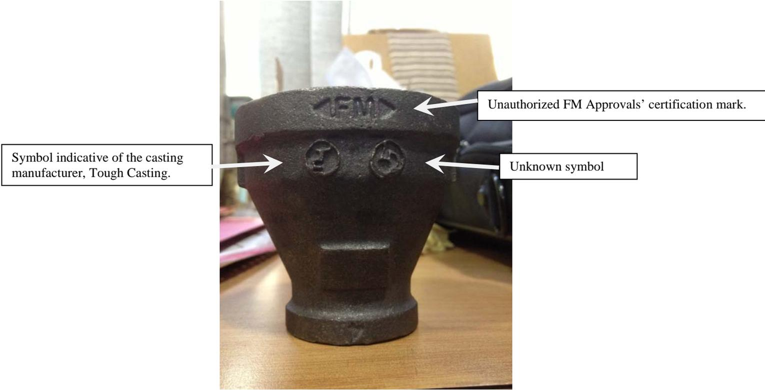
**Figure 1** – Example of the marking identifiers on the counterfeit castings.
