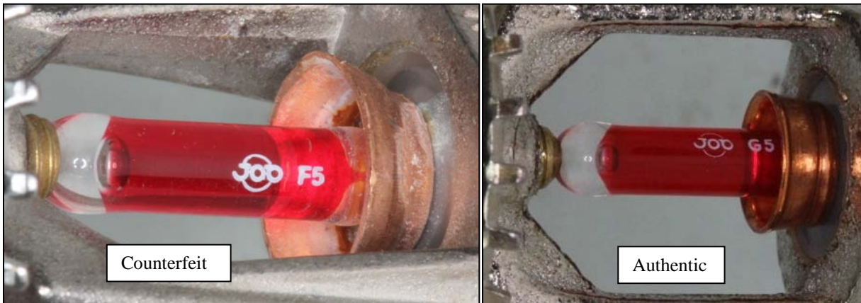
Figure 3 – Comparison of the glass bulb used in the counterfeit sprinkler (left) and an authentic Viking VK100 sprinkler (right)
