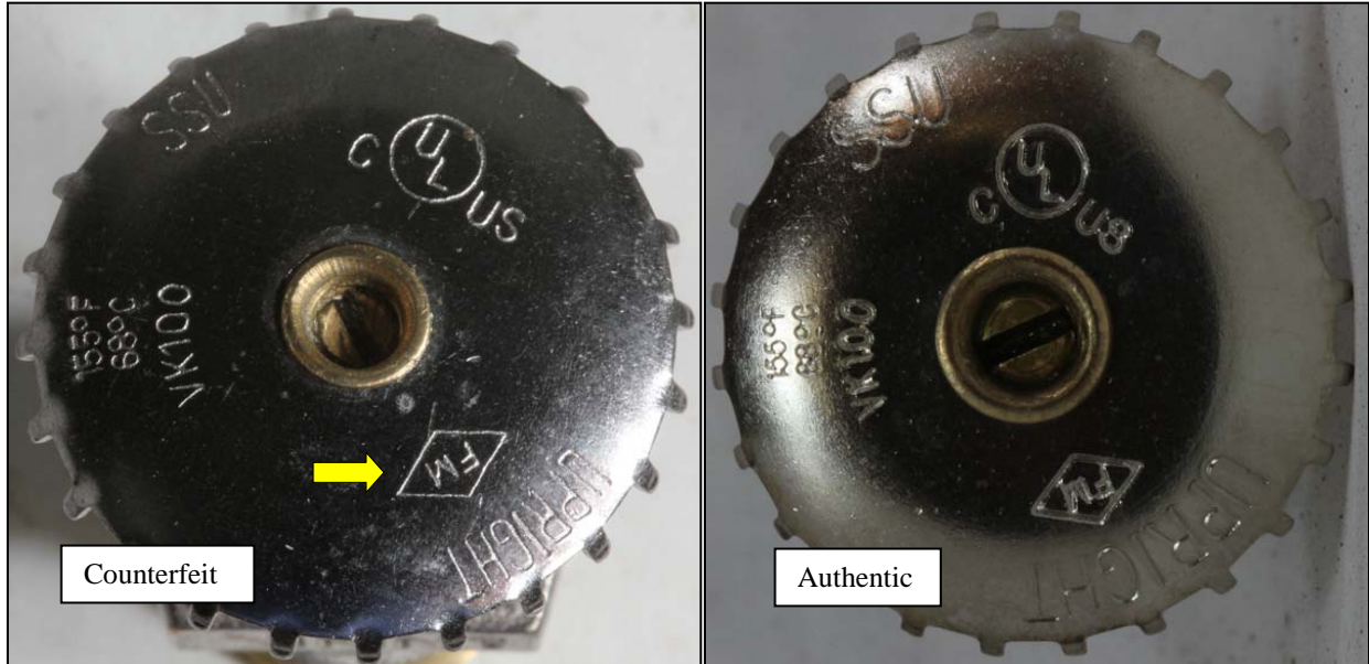
Figure 4 – Deflector markings stamped into the deflector of the counterfeit sprinkler (left) and an authentic Viking VK100 sprinkler (right)
