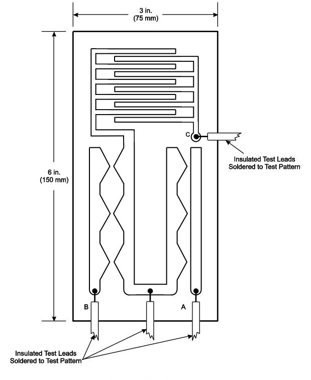
Figure B-10: Dielectric Test Pattern
