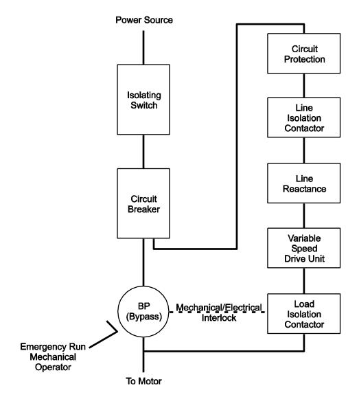
Figure B-9: Variable Speed Pressure Limiting Control
