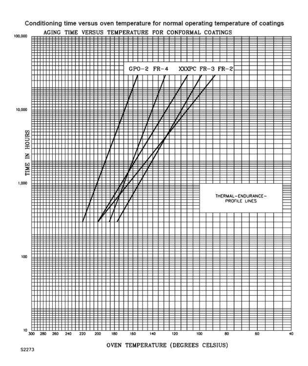
Figure B-8: Thermal Endurance Profile Curve
