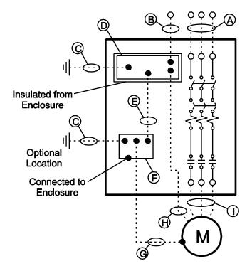
Figure B-7: Grounding/Bonding Terms
