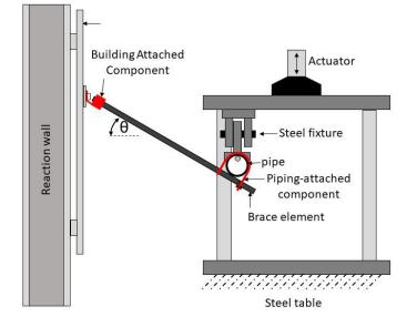
Figure 4.3.2 Test Arrangement for Assembly Testing
