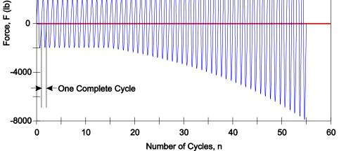
Figure 4.3.2.3 Force History Plot (Assembly Testing)
