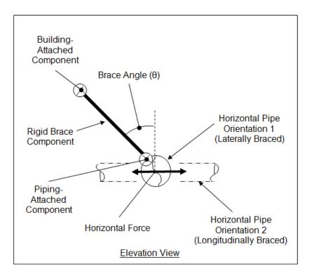
3.2.2 Figure 3.2.2A Typical Brace Layout, Horizontal Pipe
