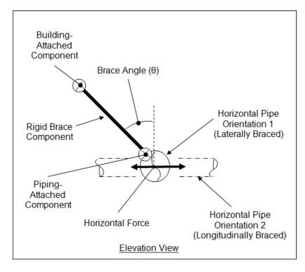
Figure 3.2.2A Typical Brace Layout, Horizontal Pipe
