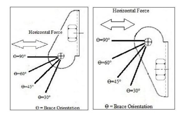
Figure 4.2.3B - Building-Attached Component with Side Attachment to Wall or Beam
