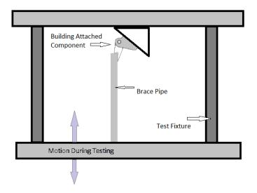
Figure 4.2 – Building Attached Subassembly, 30° Orientation
