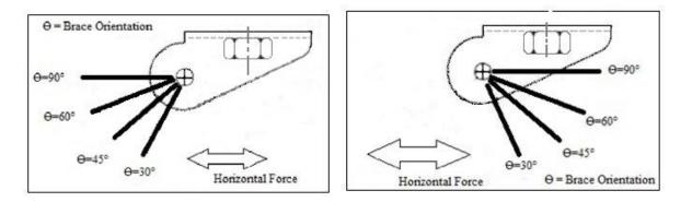
Figure 4.2.3A - Building-Attached Component with Overhead Attachment to Floor or Beam
