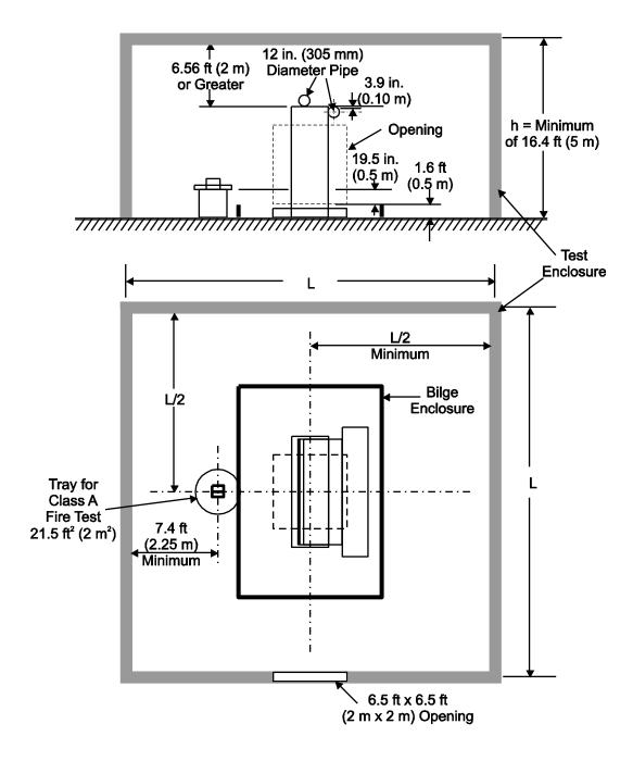
Figure C-1. Machinery and Combustion Turbine Test Enclosure
