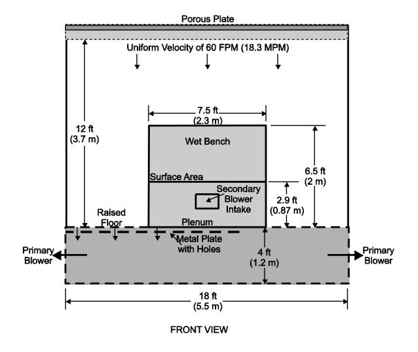
Figure D-3. Clean Room Simulation Facility - Front View
