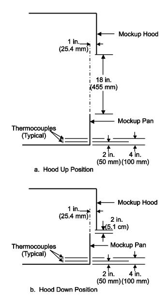
Figure F-4. Schematic of Hood Up and Down Positions
