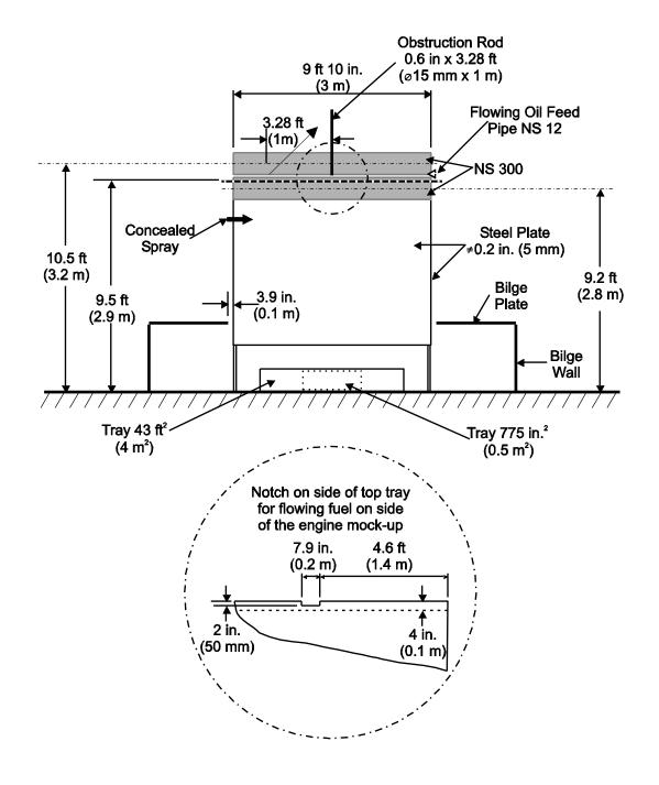
Figure C-3. Machinery and Combustion Turbine Mockup Unit (continued)
