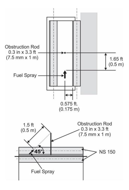
Figure K-4. Fire Test K.7.2, Position of Fuel Spray Nozzle and Obstruction Rod
