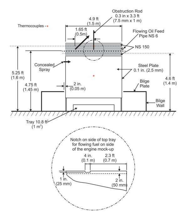
Figure K-3. Machinery and Combustion Turbine Mockup Unit (Continued)
