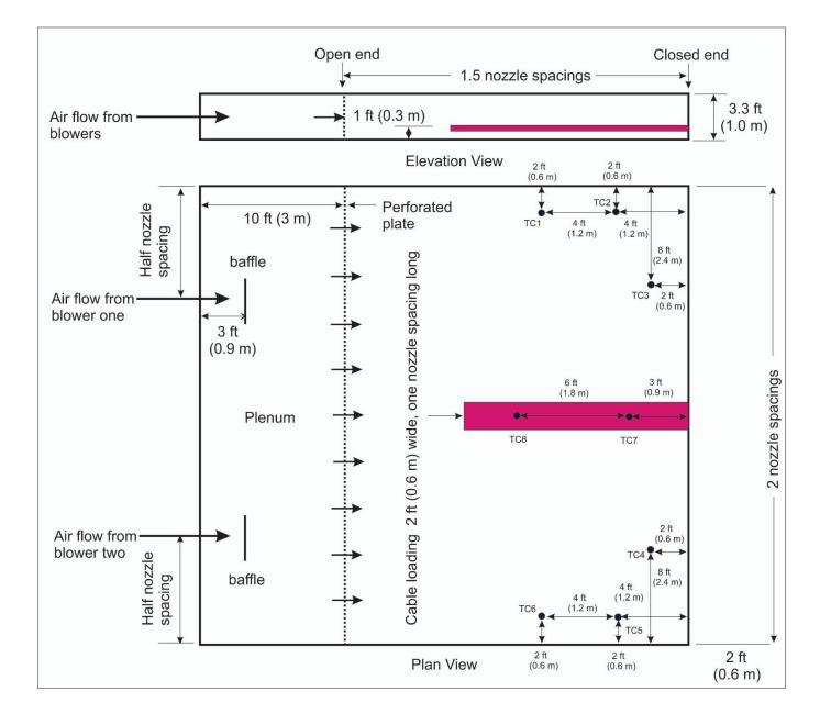
Figure J-5. Thermocouple Location Map.
