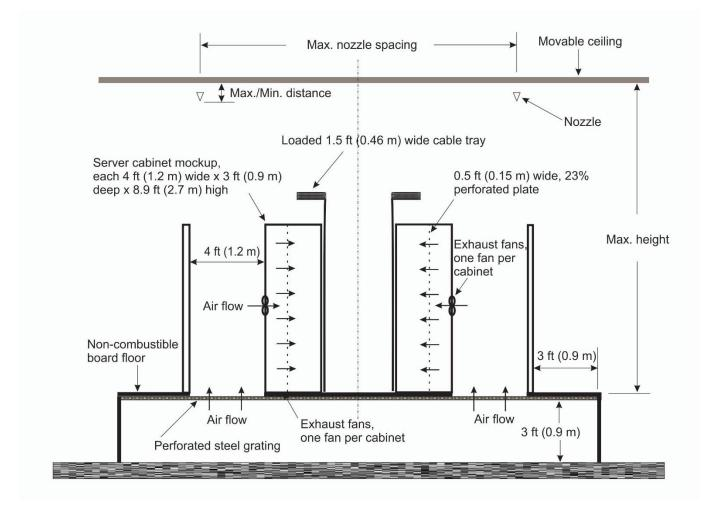
Figure I-2. Test Configuration in Elevation View.
