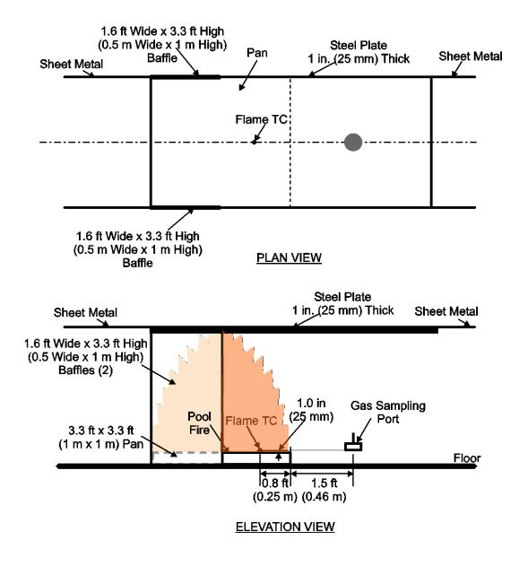
Figure A-3. Fire Source Configuration and Instrumentation for Shielded Pool Fire Testing
