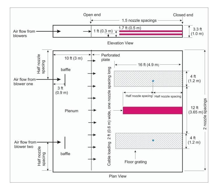
Figure J-3. Test J.5.2.3 Configuration Shown with Area of Coverage Nozzle Layout.
