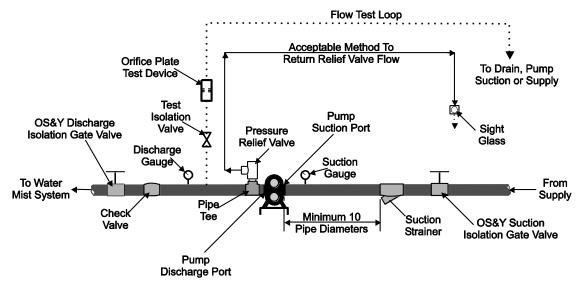
Figure 4.31 Typical Water Mist System Pump Piping and Fittings
