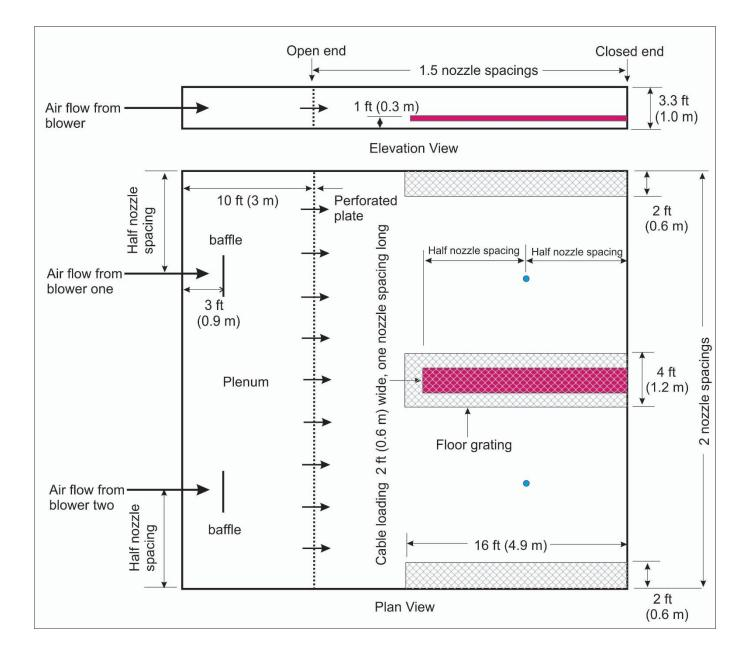
Figure J-2. Test J.5.2.2 Configuration Shown with Area of Coverage Nozzle Layout.
