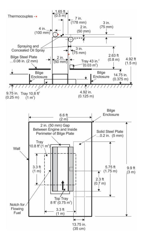
Figure K-2. Machinery and Combustion Turbine Mockup Unit
