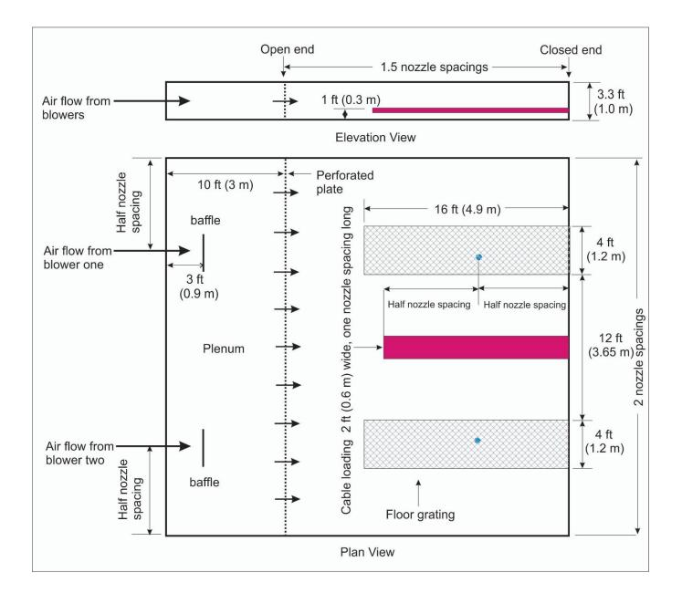
Figure J-1. Test J.5.2.1 Configuration Shown with Area of Coverage Nozzle Layout.
