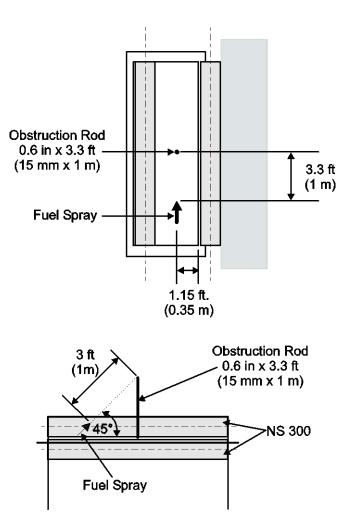
Figure C-4. Fire Test C-3-2, Position of Fuel Spray Nozzle and Obstruction Rod
