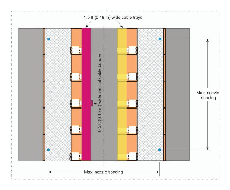
Figure I-3. Cable Fire Test Configuration.
