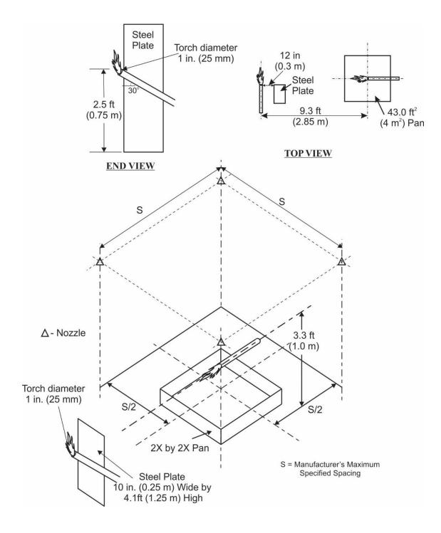
Figure E-10. Spray Fire Arrangement for Fire Scenario E.3.6
