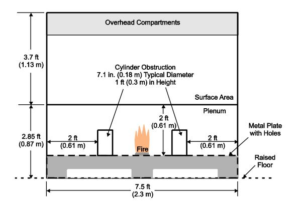
Figure D-5. Wet Bench Test Apparatus for Plenum Fire Subsurface Testing with Obstructions - Front View
