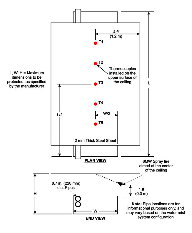
Figure G-6. Test Setup for the Obstructed 6MW Spray Fire Scenario in the Press Pocket Space
