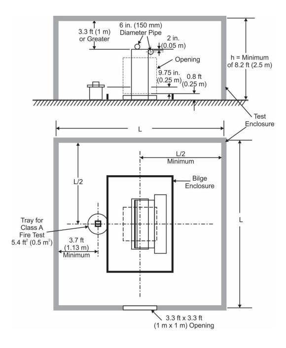
Figure K-1. Machinery and Combustion Turbine Test Enclosure
