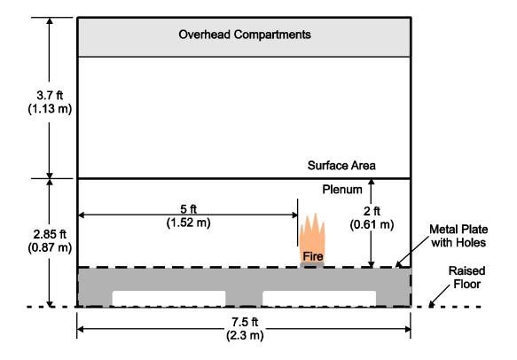
Figure D-6. Wet Bench Test Apparatus for Plenum Fire Subsurface Testing without Obstructions - Front View
