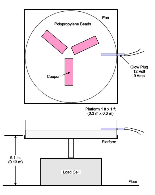
Figure D-8. Polypropylene Pool Fire for Wet Bench Fire Testing
