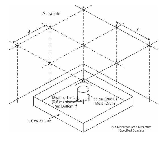
Figure E-9. Shielded Pool Fire for Fire Scenario E.3.5
