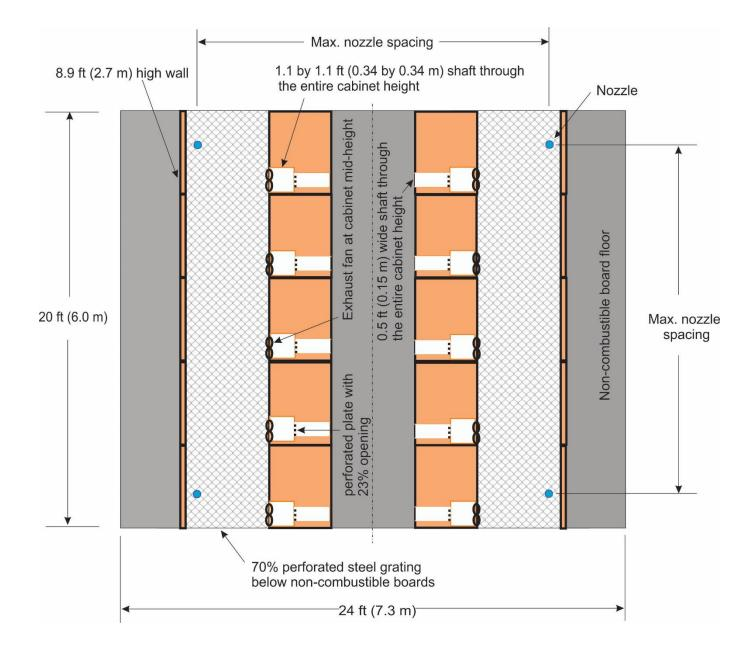
Figure I-1. Test Configuration in Plan View.
