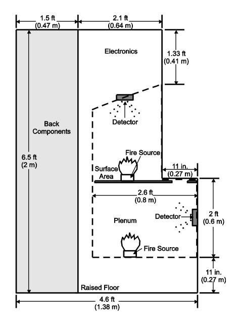
Figure D-4. Wet Bench Test Apparatus - Side View
