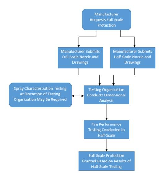
Chart K.2: Half-Scale Testing Process Flow Diagram
