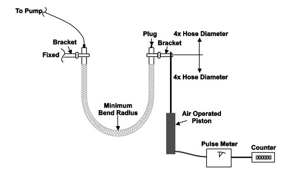
Figure N-1. Test Apparatus for Fatigue Test
