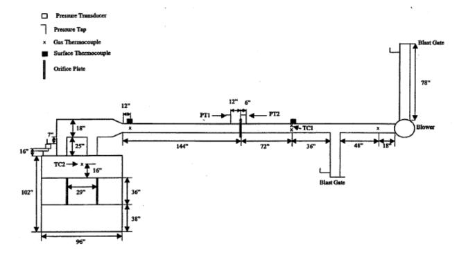
Figure H-1. Sketch of Example Mockup Arrangement for Fume Hood (Front View)
