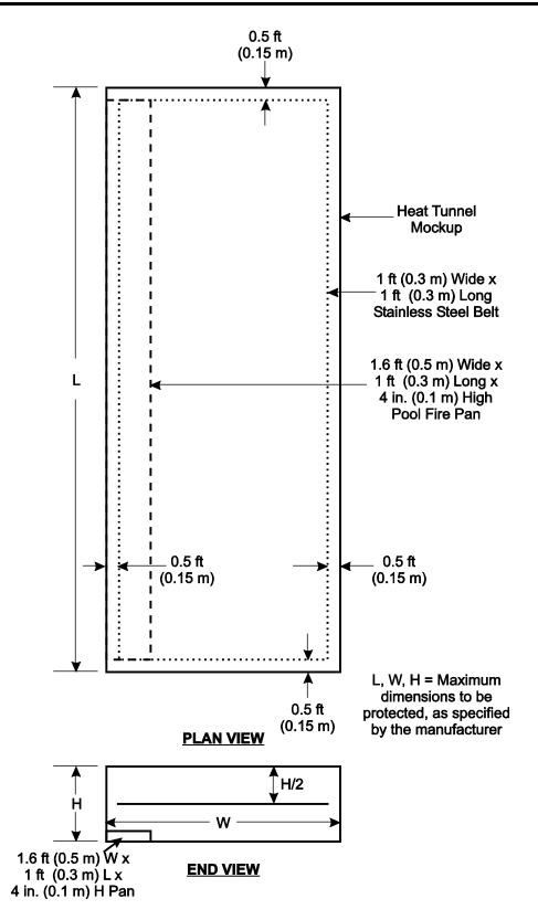
Figure G-3. Press Heat Tunnel Mockup
