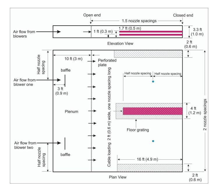
Figure J-4. Test J.5.2.4 Configuration Shown with Area of Coverage Nozzle Layout.
