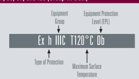
Ambient temperature ranges other than standard (-20°C < Ta < +40°C) must be marked. Additional EU marking per 2014/34/EU (ATEX)
