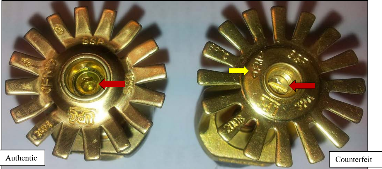
Figure 2 – Deflector and deflector markings on an authentic Angus Model S sprinkler (left) and on the counterfeit sprinkler (right)
