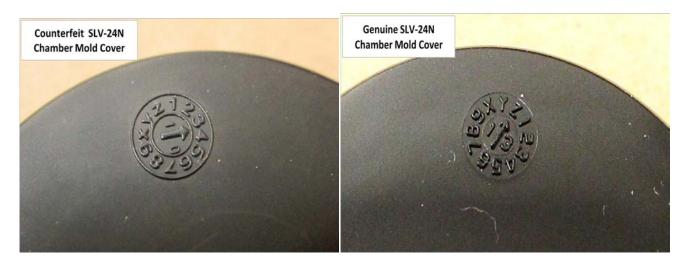
Counterfeit SLV-24N Chamber Mold cover on the left, genuine on the right.
