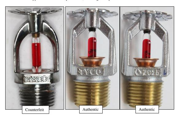
**Figure 1.** Comparison of a sprinkler found bearing the counterfeit FM Approvals mark and what appears to be a pendent style deflector (left) and an authentic Tyco TY3251 (middle and right)
