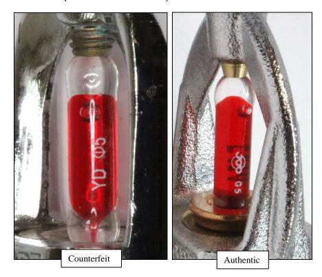
Figure 6. The different bulbs used in the counterfeit Globe sprinklers (left) and authentic Globe sprinklers (right)
